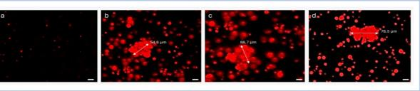
Coagulation in the in vitro experiment. (a) solution containing only MPs at 500 mg/L; (b) MPs solution (500 mg/L) added with microencapsulated ASX (1× concentration); (c) MPs solution (500 mg/L) added with empty microcapsules (1× concentration); (d) MPs solution (500 mg/L) added with starch (1× concentration). Scale bars: 20 μm.
